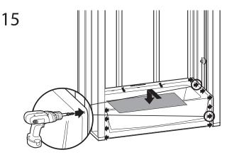
Pre-drill horizontal flanges along top of base section and fasten into each corresponding stud. Pre-drill both (vertical) side flanges and fasten to side studs 8" (200mm) on center. Place cardboard to protect surface.
