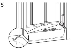
Level and mark all sides. Front apron should be firmly on the floor.
