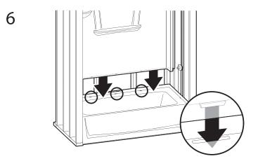
Lift and place the back wall, making sure locking tabs are engaged.
