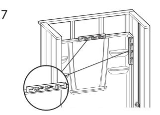
Level back wall vertically. Shim if necessary.
