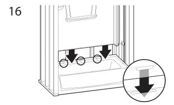
Lift and place back wall, making sure locking tab is engaged.
