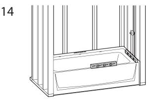
Level lengthwise and widthwise using 3 ft. (915mm) level by shimming if necessary. The unit must be set level.
