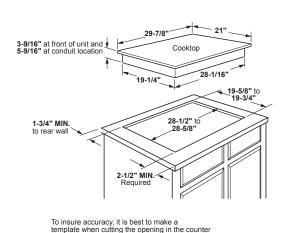
30" MIN. Clearance from countertop to unprotected overhead surface 2" MIN. Clearance from cutout to nearest vertical wall or cabinet on left side of the unit
