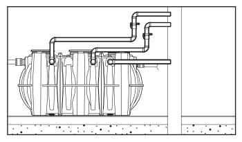
Install 3" PVC piping, connections, valves and/or hardware from the interceptor pumpout port to pumpout hook-up location (**Not included with this unit**). Maximum quantity of 6 elbow fittings per line. Max. height from static water line of interceptor to hook-up is 21 feet. Max horizontal distance from interceptor to pumper truck (including hose) is 100 feet.
