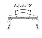
Loosen the cover adapter upper band clamp using 7/16" nut driver bit. Adjust cover adapter heights as needed. Maintain a minimum 2-1/2" insertion depth. Tighten upper band clamp to 5 -8 ft. lbs. of torque using 7/16" nut driver bit. If required, cover adapters may now be tilted up to 10° in any direction using gasket flexibility.
