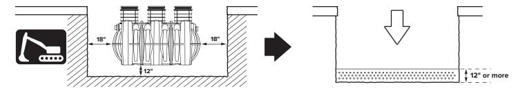
Excavate hole at least 18" larger than interceptor on all sides and 12" deeper than tank bottom. Lay a level bed of well-packed, crushed aggregate (approximately 3/4" size rock or sand, with no fines) in the base of hole.
