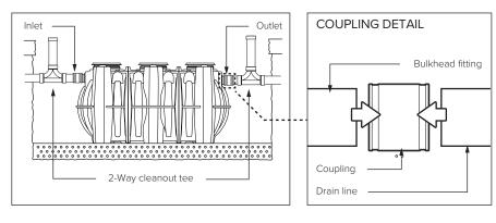
Place unit into final position and set level. Mechanically couple inlet and outlet drainage lines to unit. **Do not solvent weld.** Ensure all upstream fixtures are trapped. Vent per local code. Installation of 2-way cleanout tees to grade (by others) is recommended for buried installations.
