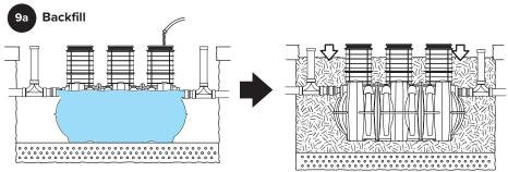
rock or sand with no fines)or flowable fill. Do not mechanically compact backfill around unit.
