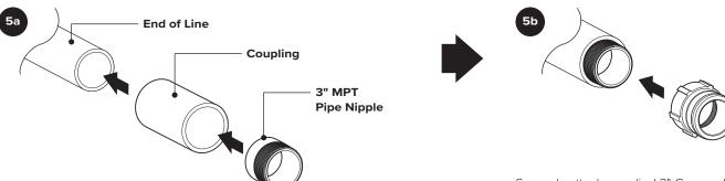
At the end of the pumpout plumbing line, install a 3" MPT pipe nipple (**Not included with this unit**) using a coupling of your choice.
