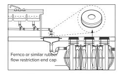
piping that discharges into the drain. See drawing for guidance. For detailed guidance on indirect connections, go to: webtools.schierproducts.com/Technical\_Data/Indirect\_Connections.pdf
