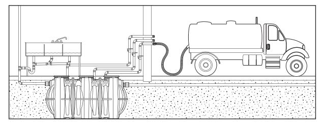
Run sinks to ensure interceptor is full of water. Attach pumper hose to 3" cam and groove fitting. Turn on pump, make sure interceptor is pumped out and inspect pumpout plumbing for leaks.
