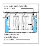
table scenarios must be installed with an anchor kit. Model GB-1500 uses model AK3 anchor kit for use with deadmen anchors.
