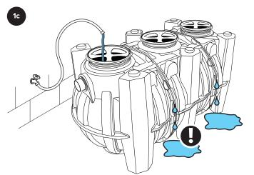
Remove covers. For base unit testing fill with water to just above the highest connection.
