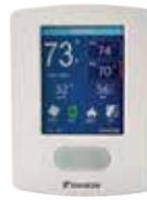
The Daikin *Adaptive Touch Controller* (ATC) is used to control FDMQ and FFQ (P1P2) indoor units with advanced and configurable control logic. The *ATC* comes in 4 different models with a built-in temperature sensor, humidity sensor, CO<sub>2</sub> sensor, and occupancy sensor. The
