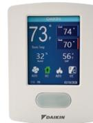
The Daikin *Adaptive Touch Controller* (ATC) is used to control FDMQ & FFQ indoor units with advanced and configurable control logic. The ATC comes in 4 different models with a built-in temperature sensor, humidity sensor, CO<sub>2</sub> sensor, and occupancy sensor.
