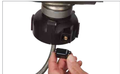
4. Remove the dust cover from the sensor.
