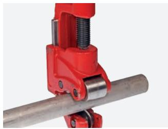
After measuring, the pipes can be cut to length using a pipe cutter designed for stainless steel, a fine-toothed handsaw or an electrical mechanical saw suitable for the pipe material. The pipe must always be cut completely through. Do not
