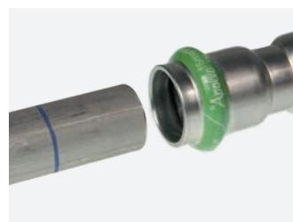
Insert the pipe end carefully into the fitting while turning and pushing it in the direction of the axis until it comes to a stroke stop in the socket. The patented sealing element design also functions as a sealing element detection solution. This means
