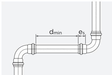
To optimise installation time, you may assemble a number of connections first and then press the various pipe connections, one after the other.
