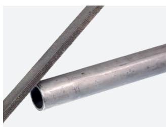
Pipe ends must be thoroughly deburred on the inside and the outside once they have been cut to length. This is necessary to avoid any damage to the sealing element when inserting the pipe into the press fitting. A file or hand deburrer or an
