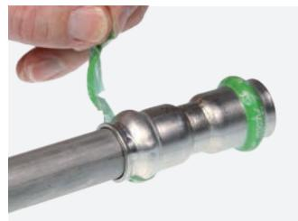
As a visual indication that the connection has been pressed, the Visu-Control® foil should be damaged. Remove the foil as an indication that the connection has been pressed and checked.
