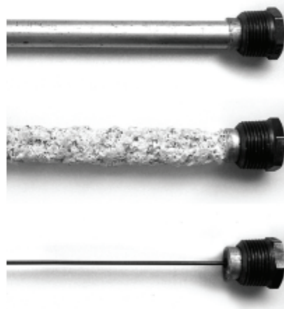
Figure 29 - Anode Rods from new (top) to partially depleted (middle) to fully depleted (bottom).
