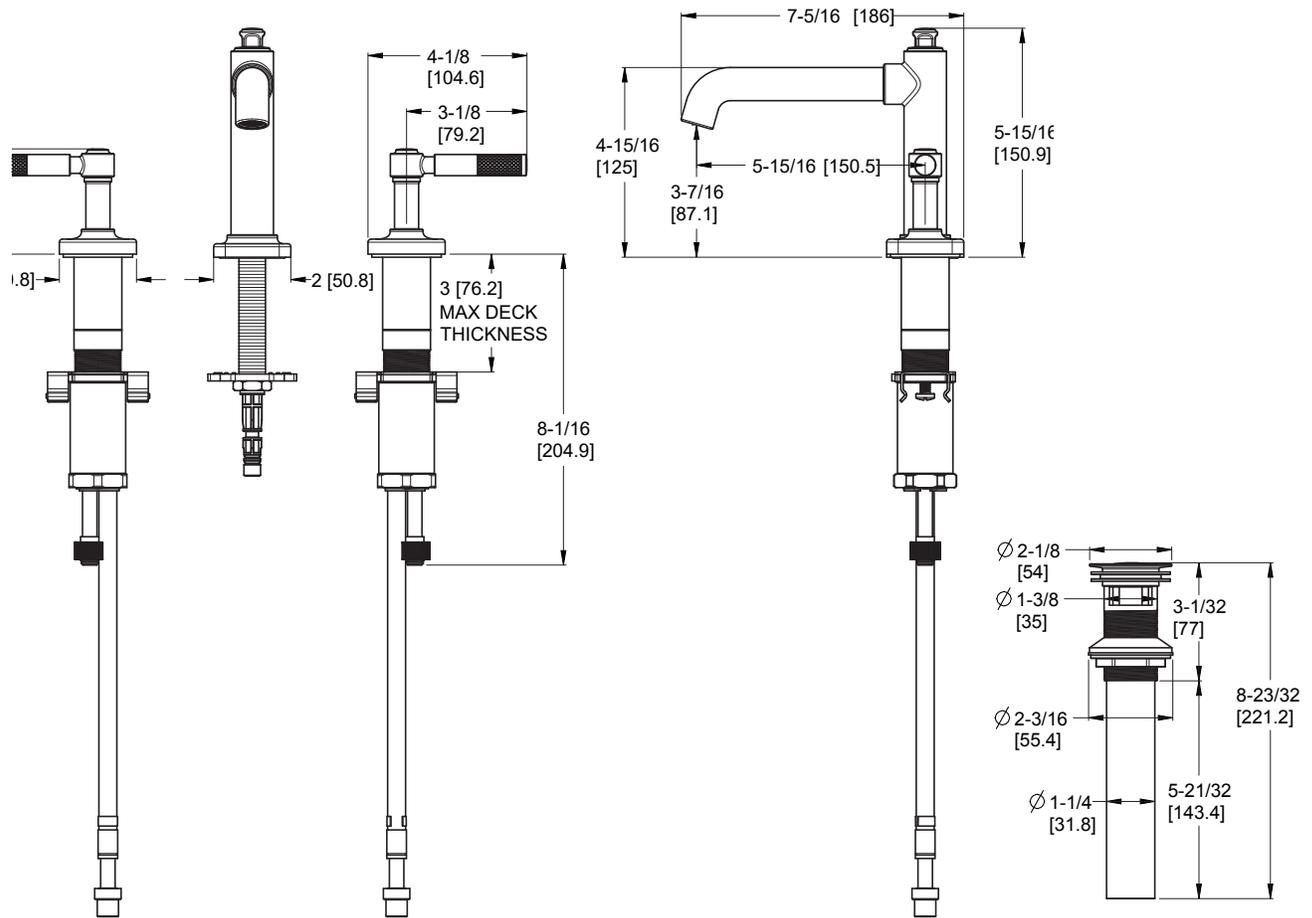
Ø1-1/4 Min to Ø1-1/2 Max. Deck Hole Openings
