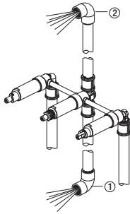
4. For tub and shower combinations, turn on the hot and cold water supply lines, allowing water to flow from the tub spout outlet (1) until all debris is cleared from the line. Check all connections for leaks.
