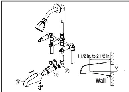
6. Wrap thread sealant tape around the pipe threads of the tub spout outlet (1, not included) in a clockwise direction, as shown. Connect the tub spout outlet pipe (the tub spout outlet pipe should project 1-1/2 in. to 2 1/2 in. from the finished wall) to the lower pipe elbow (2, not included). Tighten the elbows and tub spout outlet pipe connections with the strap wrench. Tighten the elbow and tub spout (3) outlet pipe connections with a strap wrench.
