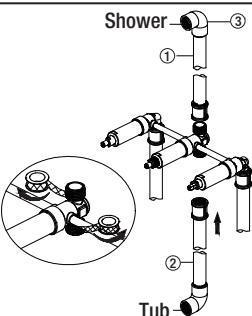
3. Wrap thread sealant tape around the valve body threads in a clockwise direction, as shown. Connect the shower (1) and tub outlet pipes (2) to the valve body. Connect the pipe elbows (3) (not included) to the ends of both pipes, and tighten with a wrench.
