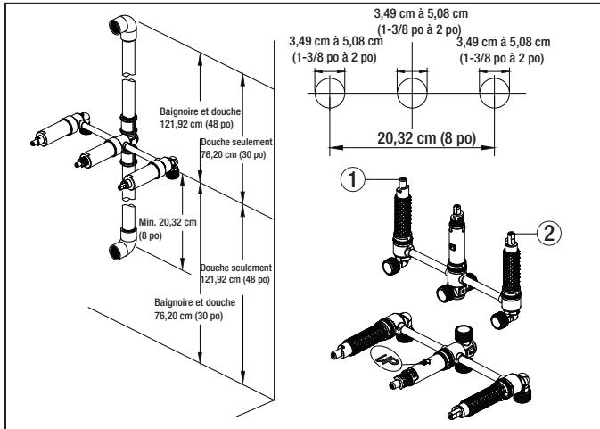
1. Shut off the water supply to the tub and shower. Verify that the hole sizes and positions of the holes in the wall are correct.
