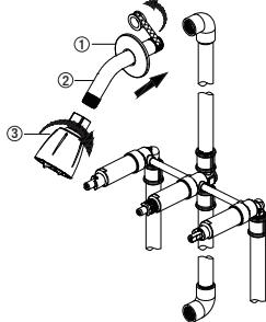
5. Insert the long end of the shower arm (2) through the shower flange (1), then wrap thread sealant tape around the long end of the shower arm (2) in a clockwise direction, as shown.
