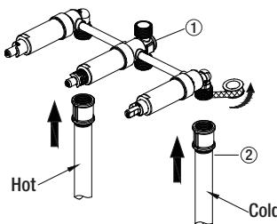
2. Wrap thread sealant tape around the valve body (1) threads in a clockwise direction, as shown. Thread the waterline (2) to the valve body (1), and tighten with a wrench.
