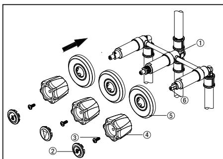
7. Position the flanges (5) on the valve body (1). Attach the handles (4) to the stems (6), and secure them with the screws (3). Use a Phillips screwdriver to tighten the screws (3). Attach the indexes (2).
