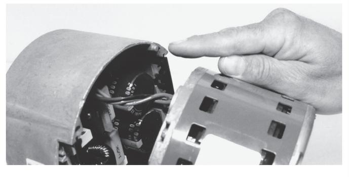
5. For proper motor cooling, it is important that the motor be mounted the same as the original, as far into the blower as practical.
