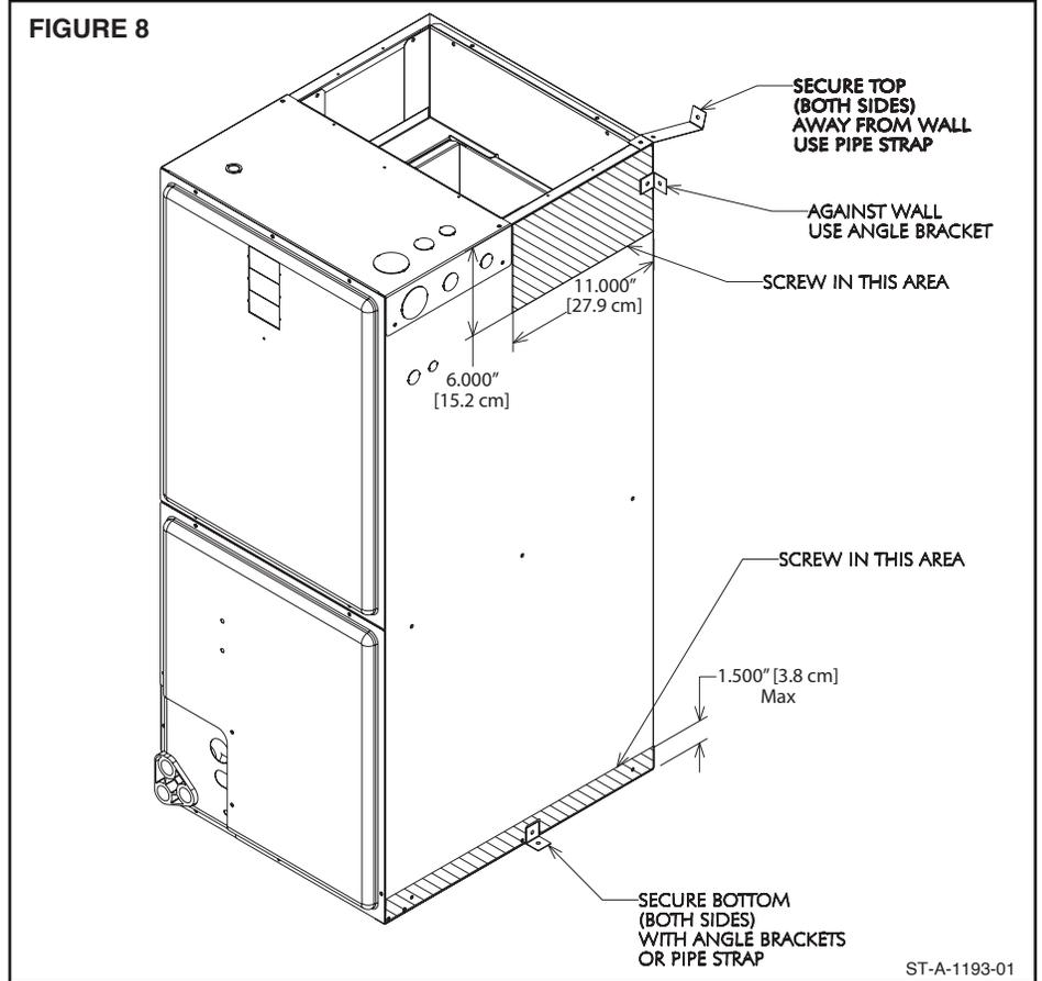
16ga thick angle brackets one on each side. Attach brackets with No. 10 self-tapping  $\frac{1}{2}$ " [13mm] long screws to air handler and use  $\frac{5}{16}$ " [8 mm] lag screws  $1\frac{1}{2}$ " [38 mm] long to wall stud. Secure bottom of unit with two 16ga "L" brackets with No. 10 self-tapping  $\frac{1}{2}$ " [13 mm] long screws to air handler and use  $\frac{5}{16}$ " [8 mm] lag screws  $1\frac{1}{2}$ " [38 mm] long to floor.
