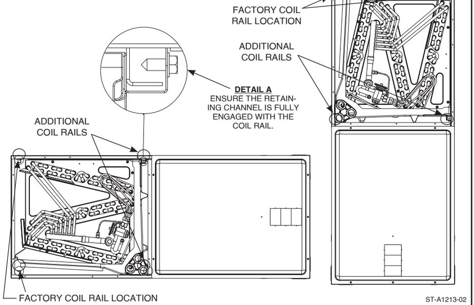
**FIGURE 7****INDOOR COIL AND DRAIN PAN DETAILS**
