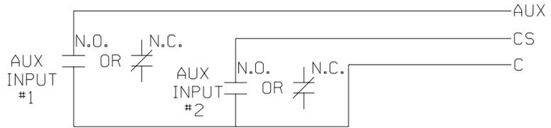
NOTE: EITHER A NORMALLY-OPENED (N.O.) OR NORMALLY-CLOSED (N.C.) ACCESSORY CAN BE ATTACHED TO AUXILIARY INPUTS 1 AND/OR 2. SELECT CONFIGURATION (N.O. OR N.C.) AT THE ECONET™ CONTROL CENTER.
