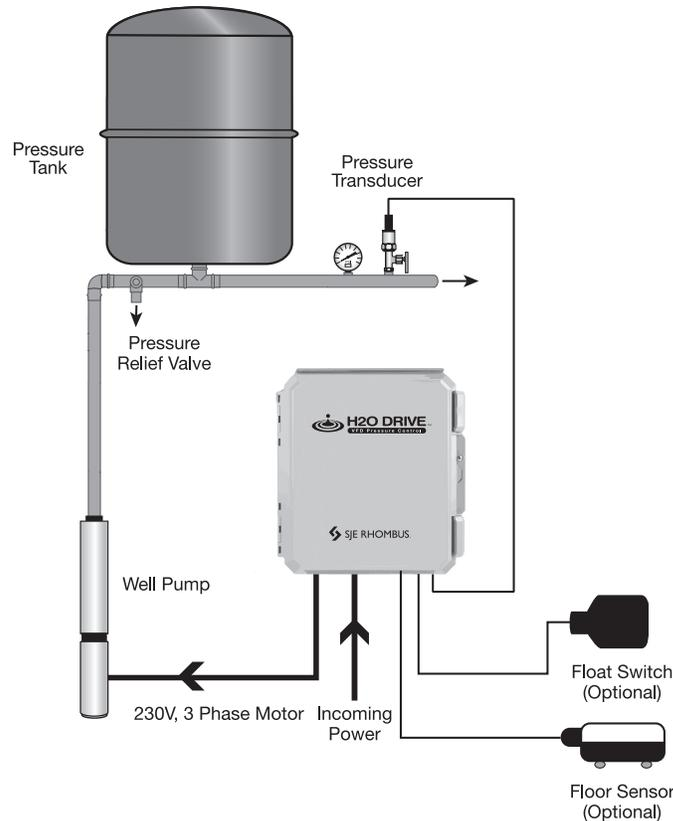
**Note: For use in clean water pressure control applications. Not for use with sewage pumps.**
