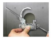
7. Press the release pin and open the bracket. Load the flexible hose at the appropriate position. Securely fasten the gate of the center bracket from right to left.
