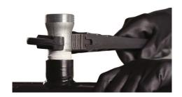
4. Use a pipe wrench to connect the flexible hose to the inlet nipple. Torque range should be a minimum of 50 to a maximum of 58 ft-lbs.
