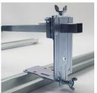
6. Tighten the wing bolts to secure the end brackets onto the hat furring channels. The recommended torque is 1.40–1.48 ft-lbs (190-200 cN • m).
