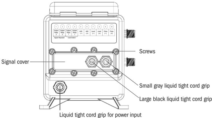
**⚠️ CAUTION** Signal cables must be UL, cUL AWM Style 2464 approved with conductors between 28 AWG and 18 AWG. Jacket diameter for small liquid tight must be 0.064" to 0.210". Jacket diameter for large liquid tight must be 0.114" to 0.250".
