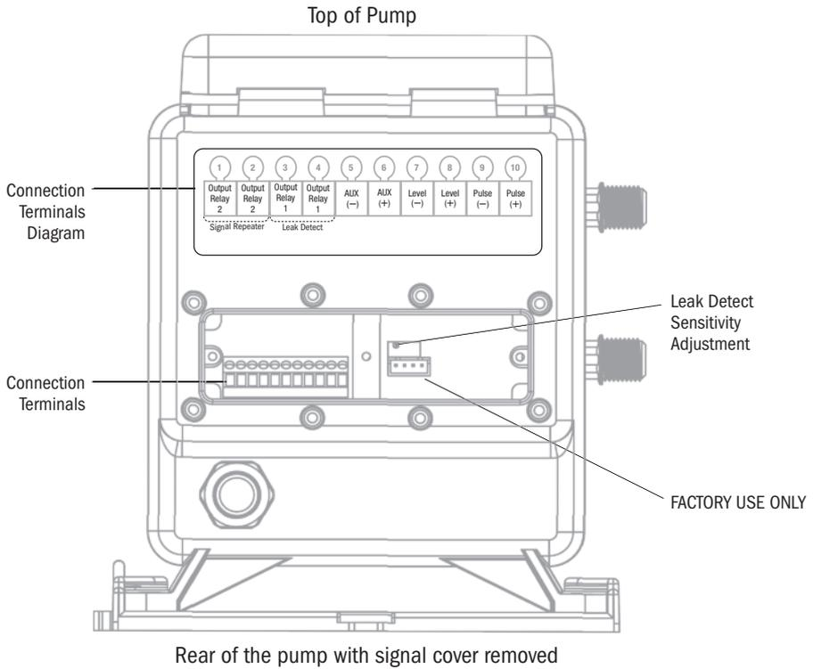
**⚠ CAUTION** If connecting a shielded signal cable to the pump, ensure that the shield wire is properly grounded on the controller (non-pump) side.
