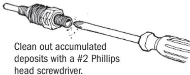
Periodic inspection and cleaning of the point of injection will maintain proper pump operation and provide maximum tube life.
