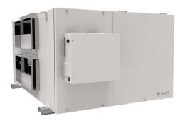
The SHR 1200 Commercial Heat Recovery Ventilation system (HRV) complements today's tight buildings. Fantech Heat Recovery Ventilators (HRV) are designed to supply air into a building while exhausting an equal amount of contaminated air to the outside. The aluminum heat exchanger core transfers sensible energy between air streams resulting in tempering of the supply air and reduced loads on the HVAC system.
