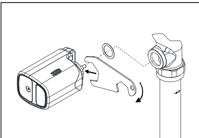
Place the supplied valve gasket onto the unit as shown. Use one hand to raise the unit to the handle port of the flush valve and use the other hand to rotate the unit's valve nut to begin engaging the threads of the valve body. Use the supplied wrench to tighten the E-Z Flush unit securely to the valve body.
