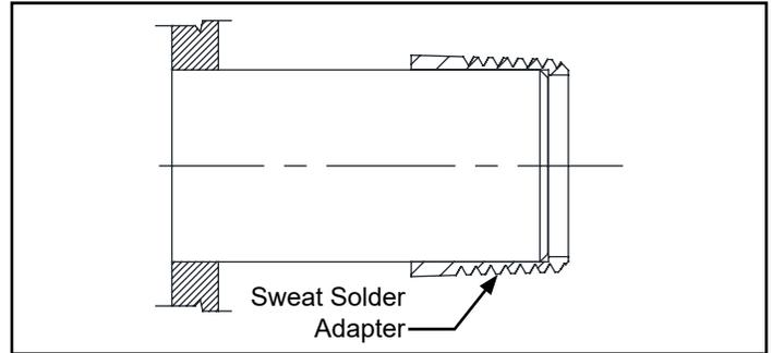
3. Measure distance from finished wall to first thread of sweat solder adapter. If necessary, cut chrome cover tube this length.
