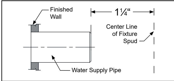
2. Slide threaded sweat solder adapter onto water supply pipe until shoulder stops on end of pipe. Then sweat-solder the adapter to water supply pipe.
