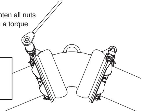
**NOTE:** Do not use an impact wrench. Do not overtorque, or retighten. If a good seal is not achieved at the installation torque, refer to the Common Installation Problem listed on side two.
