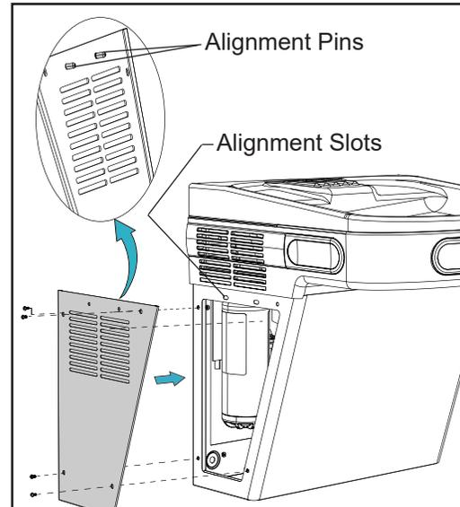
5. Once the access panel is set in place, refasten the (4) security Torx screws bits starting by hand and firmly secure each screw in place.
