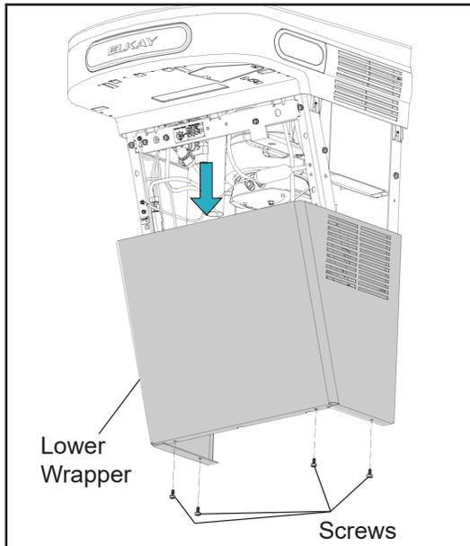
2. If you are replacing the filter, do that now with the lower wrapper removed. Refer to the Filter Replacement Instructions in Section 2, Step 3 or instruction sheet included with the replacement filter. If not, skip to the next step.
