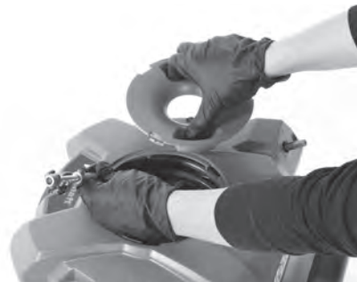
Figure 7B – Retrieve Chain Knocker/Cable
