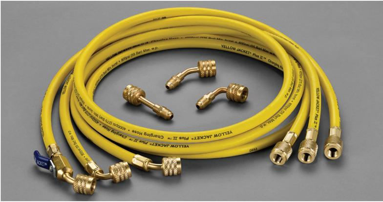
The new A2L refrigerants, R-32 and R-454A, have adopted left-handed connections for their tanks. These new refrigerants are categorized as slightly flammable, so left-handed connections were implemented to differentiate them from A1, non-flammable refrigerants. As the industry adopts these new refrigerants, **YELLOW JACKET® A2L Tank Adapters and Charging Hoses** incorporate left-handed connections so a service technician can safely charge A2L refrigerant systems.
