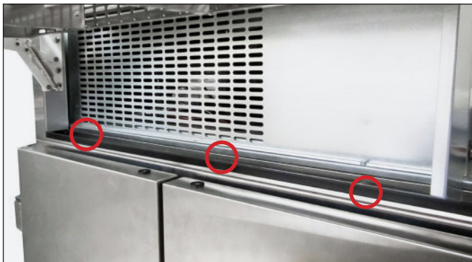
FIG. 9. Rainshield screw locations.
