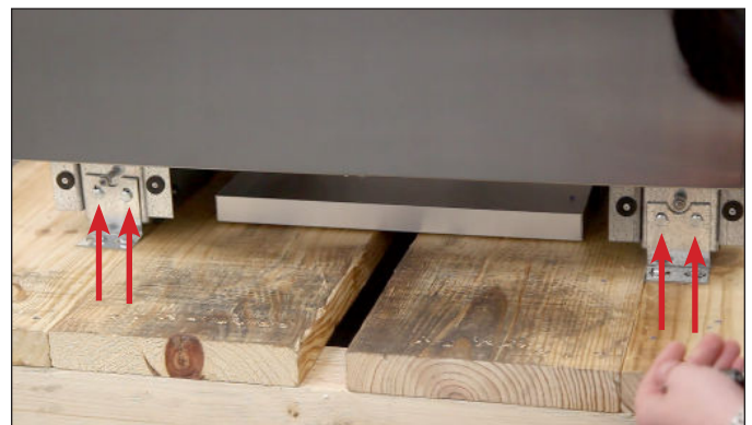
FIG. 7. Shipping bracket bolt locations.
