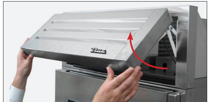
FIG. 2. Pull the rainshield open.
