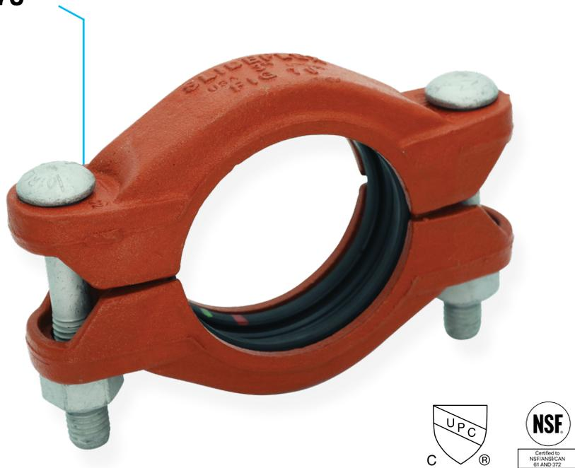
The SlideFLEX Fig 70 coupling is a flexible ready for installation coupling designed to ease assembly and reduce installation time. The patented gasket provides four separate sealing surfaces for added protection.
