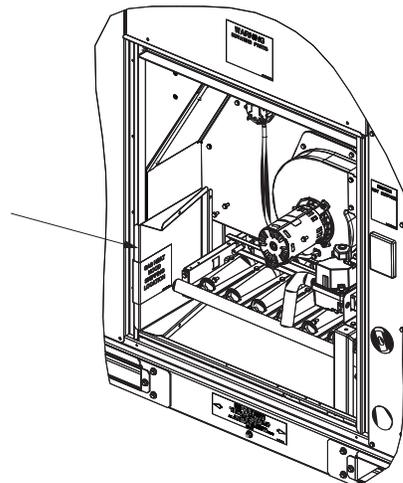
3. Install the vent hood on the gas heat panel using the screws removed in Step 1. Make sure it is properly secured to the panel.
