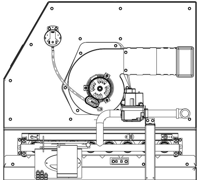
3. Remove six screws from manifold bracket. See the following figure.
