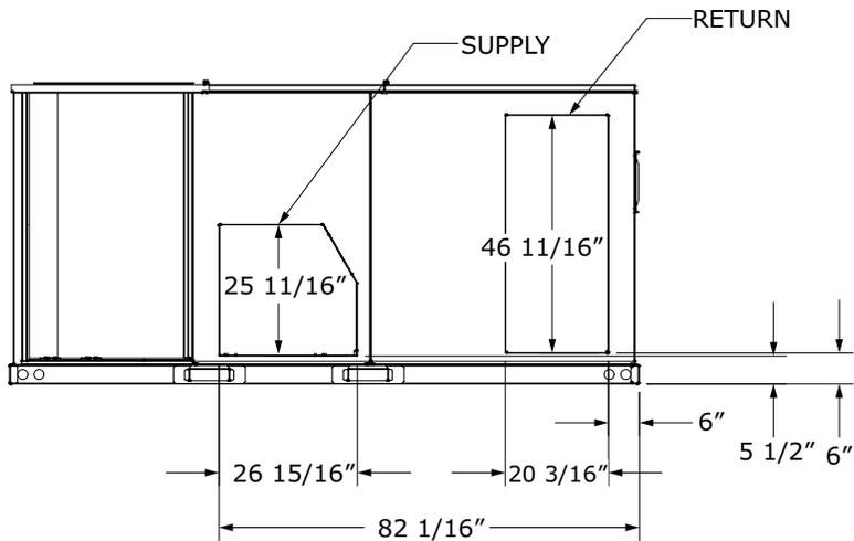
Figure 6. Cooling with optional electrical heat — roof curb
