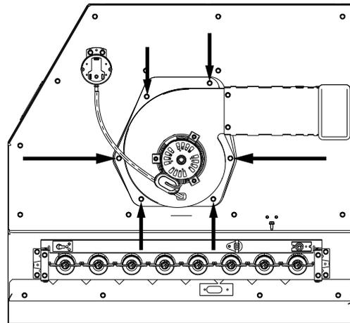
10. Install the inducer blower assembly using six screws. Confirm exhaust screen is positioned properly in the center ID post. See Figure 22.
