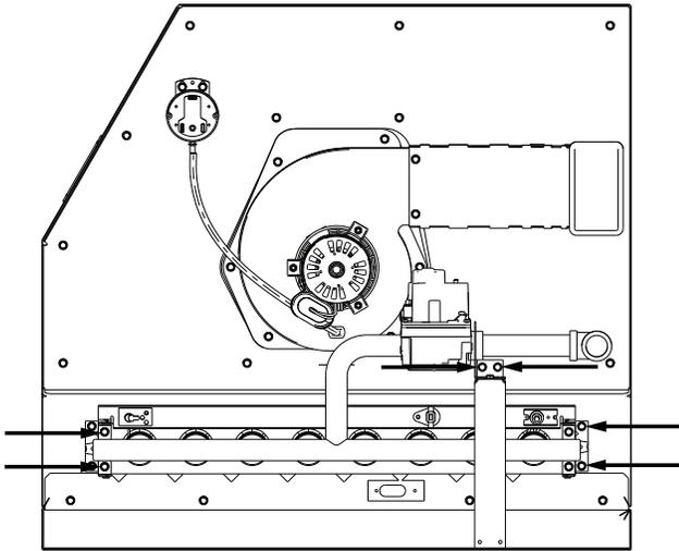
4. Remove the natural gas orifice spuds from the manifold. See the following figure.
