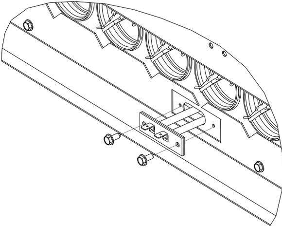
Figure 25. Location for pasting supplemental heating data label
