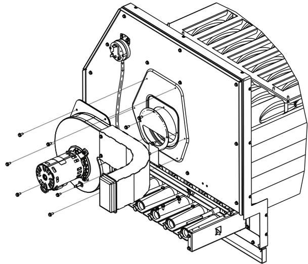
Figure 22. Remove screws from inducer blower assembly
