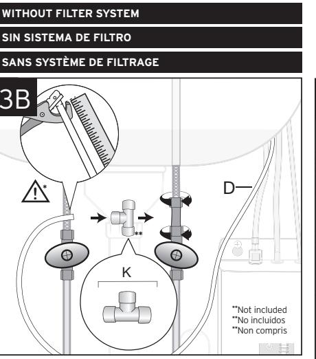
**\*NOTICE: Property Damage.** Tube runs need to form to the cabinet's contours to allow storage space with no sharp bends. Tubes need clean, perpendicular, burr-free cuts to ensure a true fit.
