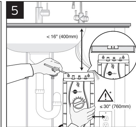
\* **NOTICE: Property Damage.** Do not plug in hot water tank until installation is complete. Tank must be located within 16" (400 mm) of instant hot water dispenser and within 30" (760 mm) or less of a standard earth (grounded) outlet. DO NOT extend plumbing or electrical lines. **Note:** An accessible location for maintenance inspection and tank replacement.
