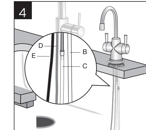
\* **NOTICE: Property Damage.** Do not pinch or break the tubes.
