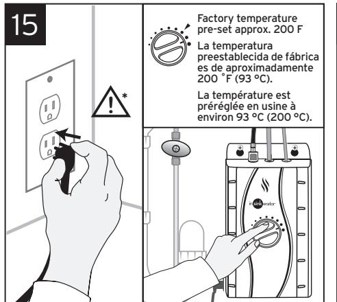
**\*NOTICE: Property Damage.** Do not use an extension lead with the instant hot water dispenser. (A standard earthed GFCI outlet within 30" (760 mm) of the instant hot water dispenser is required under the sink.)
