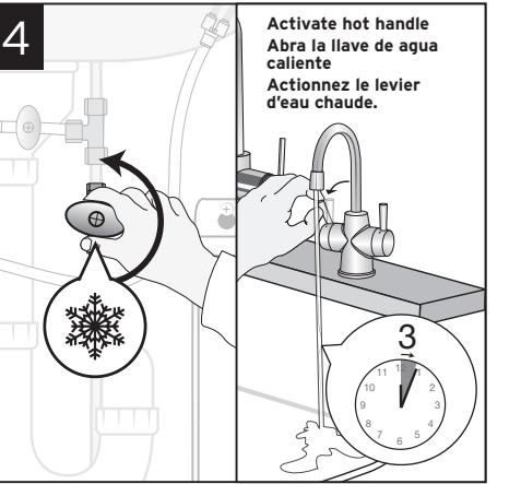
**Note:** Check all connections to ensure they are tight and that there are no leaks. To fill tank, activate handle until water is flowing. Allow water to run for 3 minutes to flush lines.
