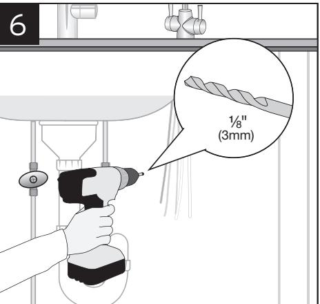
**WARNING: Personal Injury/Property Damage.** To reduce the risk associated with hazardous voltage due to an installer drilling through existing electric wiring in the area of installation: Do not install near electric wiring or water pipes which may be in path of a drilling tool when selecting the position to mount the system bracket.
