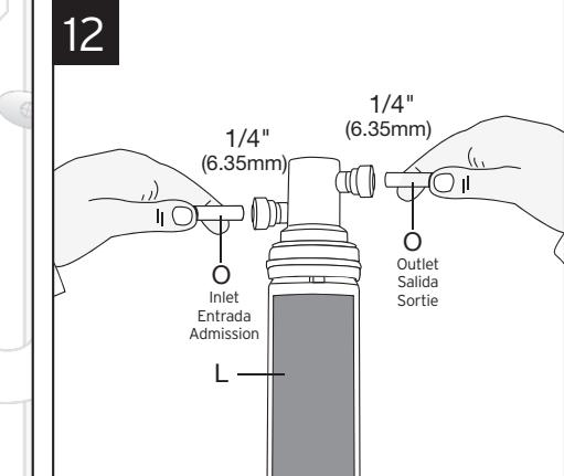
**\* NOTICE: Property Damage.** Top surface of cartridge will be flush with bottom of filter head when fully engaged.
