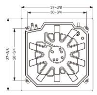
Fig. 7 —Mounting Hole Locations
