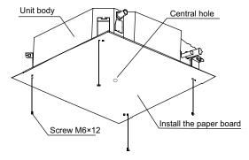
Fig. 5 —Paper Board Mounting Hole Locations
