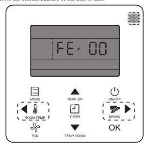
Fig. 30 —Non-Programmable Controller IDU Addressing Menu
