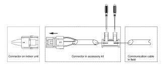
Fig. 20 — Connecting the Communication Cable to Indoor Unit to Outdoor Unit Using the Supplied Connector
