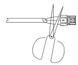
Fig. 22 —Shearing Outdoor Connector
