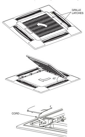
Fig. 9 —Removing Grille from Panel
