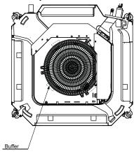
Fig. 6 —Example of Buffer Locations
