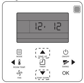
Fig. 31 —Non-Programmable Controller Setting IDU Address
