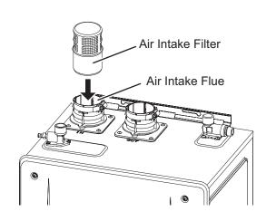
2 Continue to insert Air Intake Filter until it reaches to the base of the Air Intake Flue.
