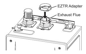
5 Spin and lock the EZTR Adapter on the Exhaust Flue as shown figure right.
