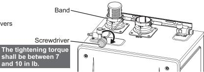
Put the EZTR Adapter the Exhaust Flue (on the right side of the unit).
