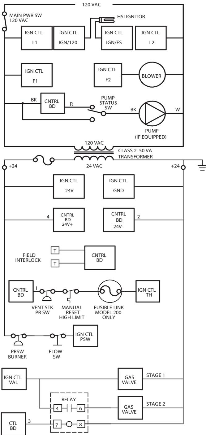
Figure 14. Logic Diagram, Hydronic Boiler
