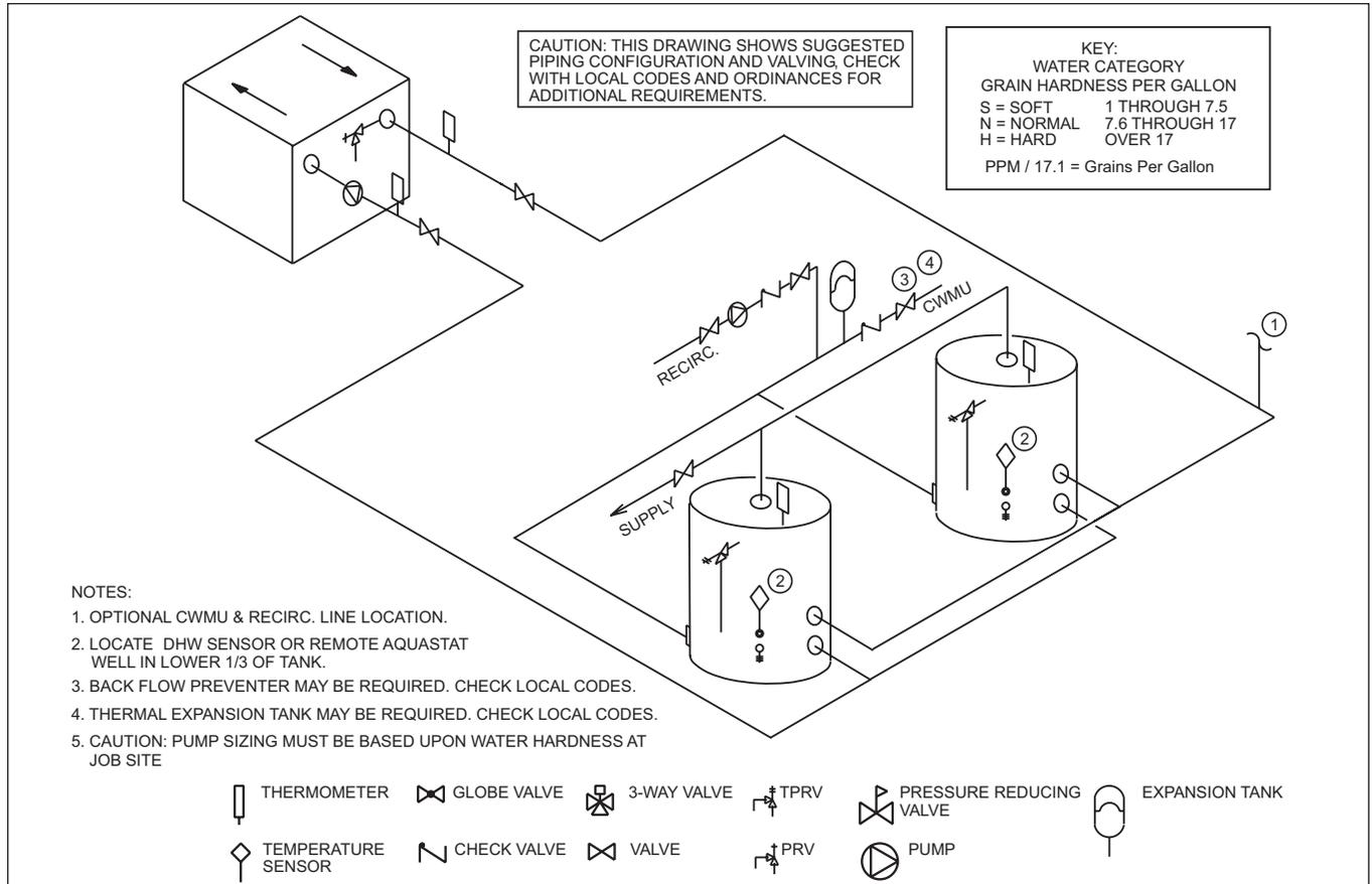
Figure 12. Water Heater Piping — One Heater, Multiple Tanks.
