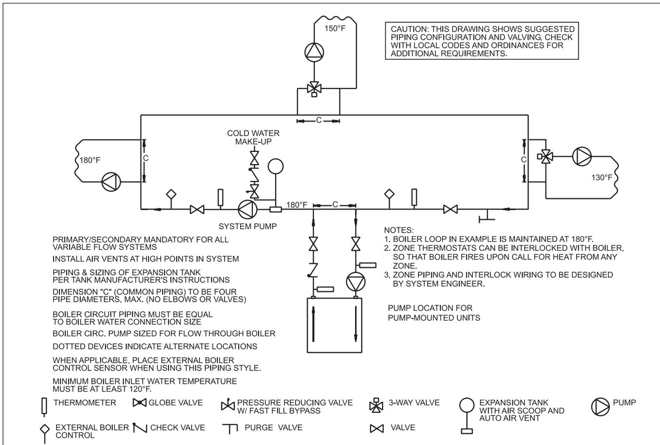
Figure 7. Hydraulic Piping — One Boiler, Multi-Temperature System.
