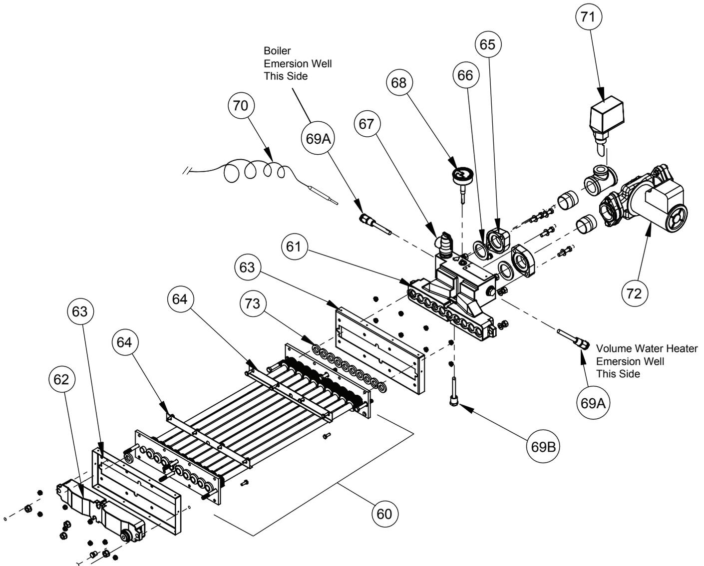
Figure 21. Heat Exchanger Components.
