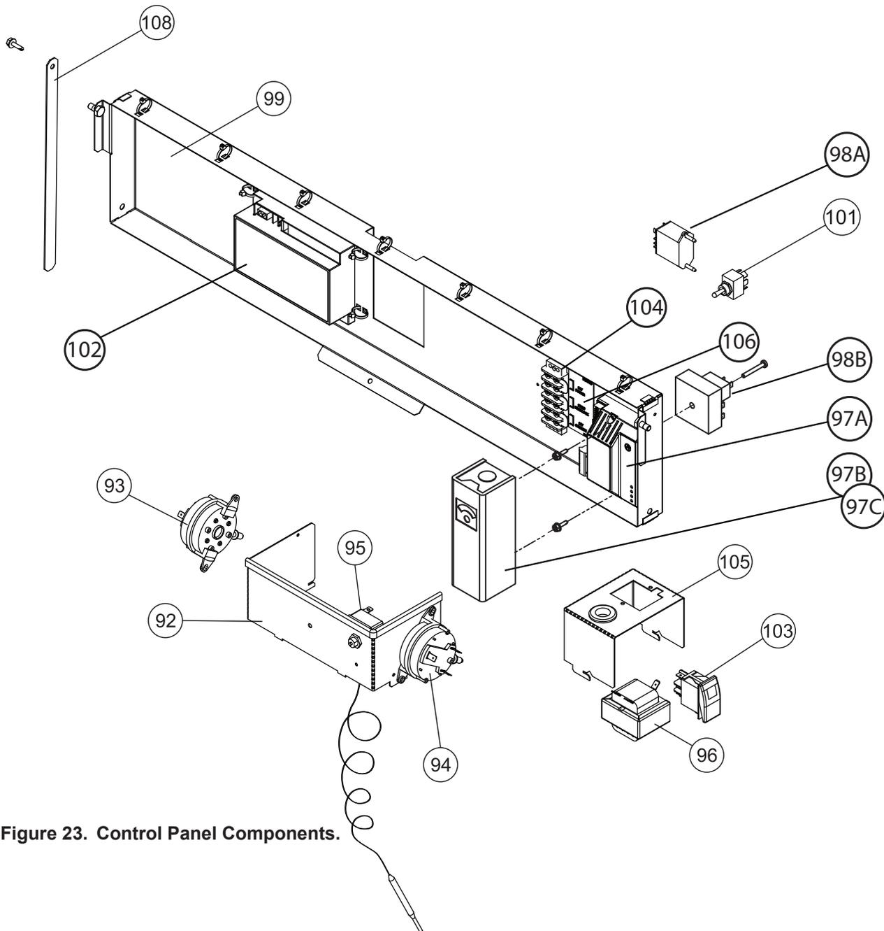
Figure 23. Control Panel Components.
