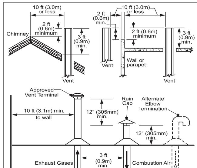
**Figure 3. Combustion Air and Vent Through Roof.**
