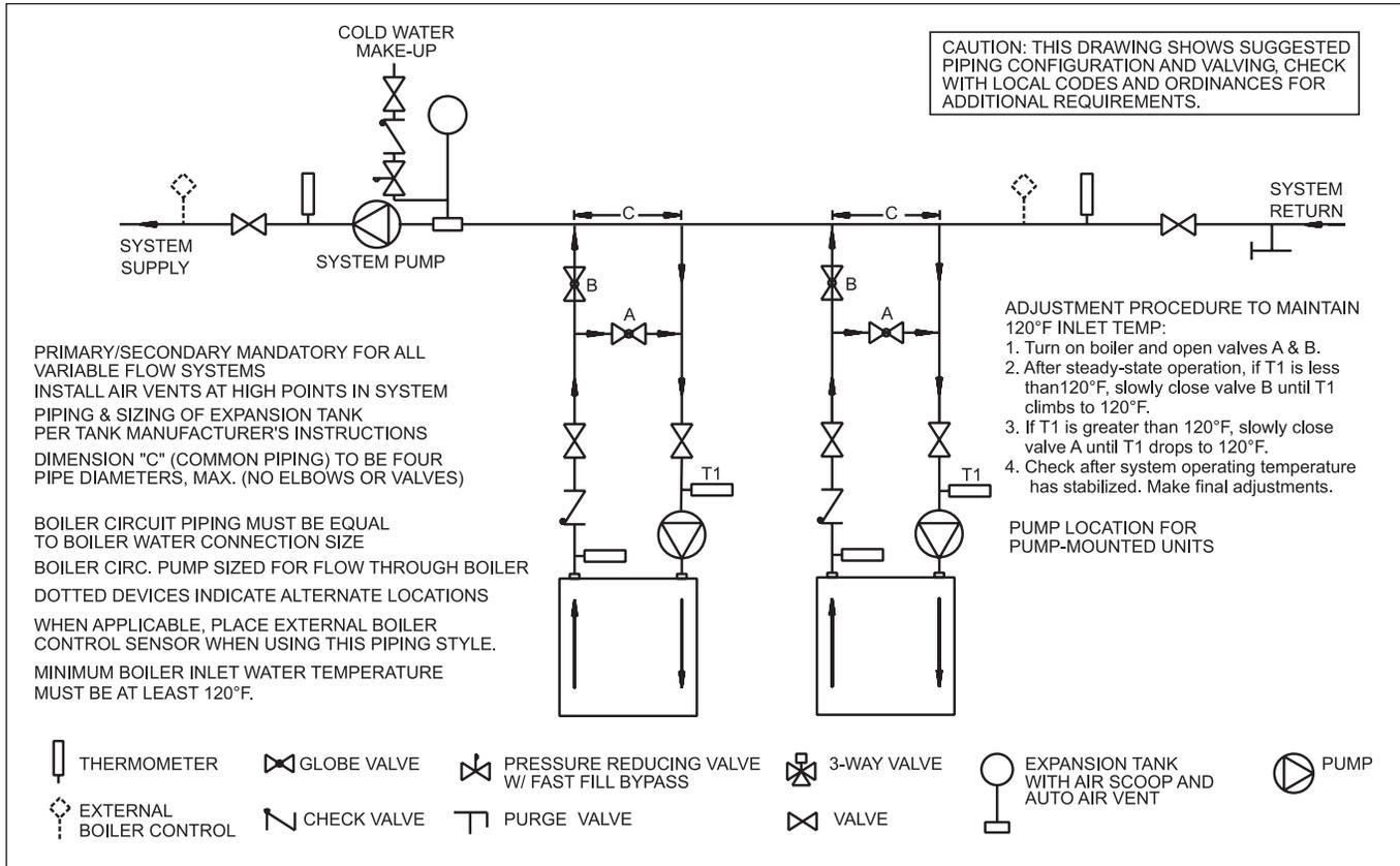
Figure 6. Hydraulic Piping — Multiple Boilers, Low Temperature System.
