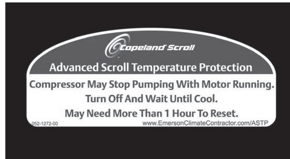
Fig. 18 — Advanced Scroll Temperature Protection Label
