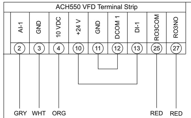
**Fig. 31 — ACH550 VFD Wiring**
