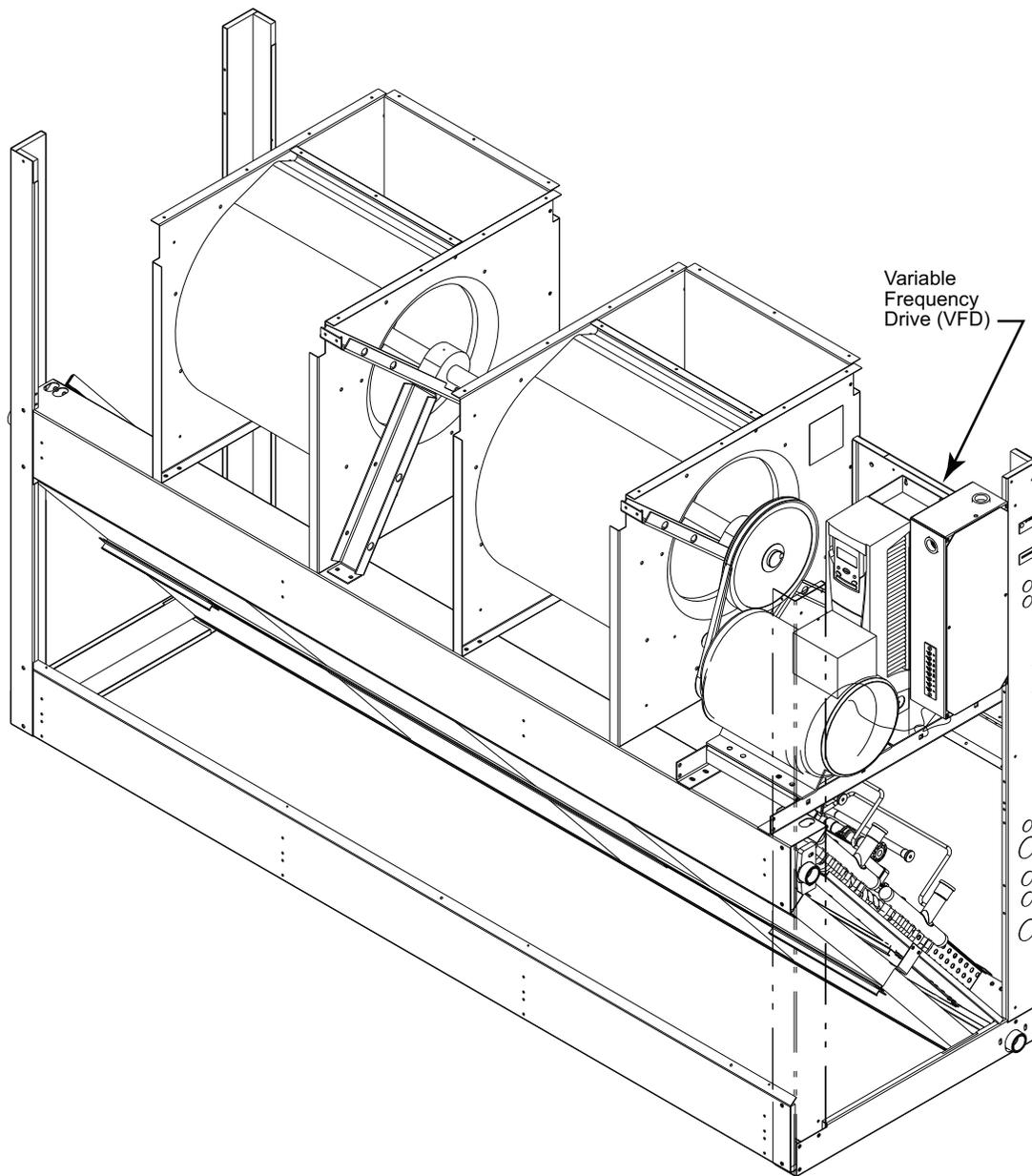
**Fig. 19 — ACH550 VFD Location for the following units: FAS150/180, FHS180 (575V only)**
