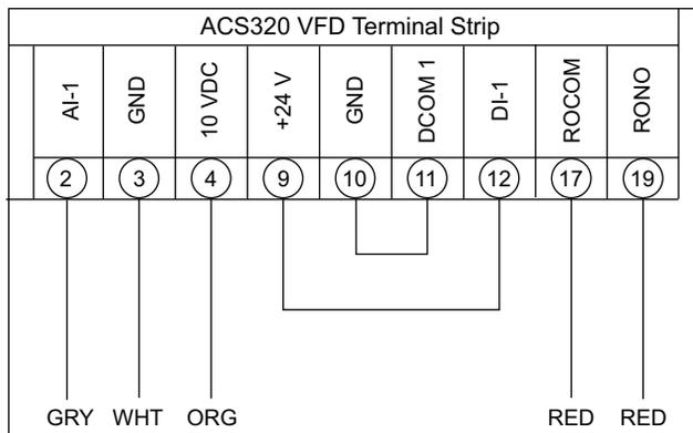
**Fig. 30 — ACS320 VFD Wiring**
