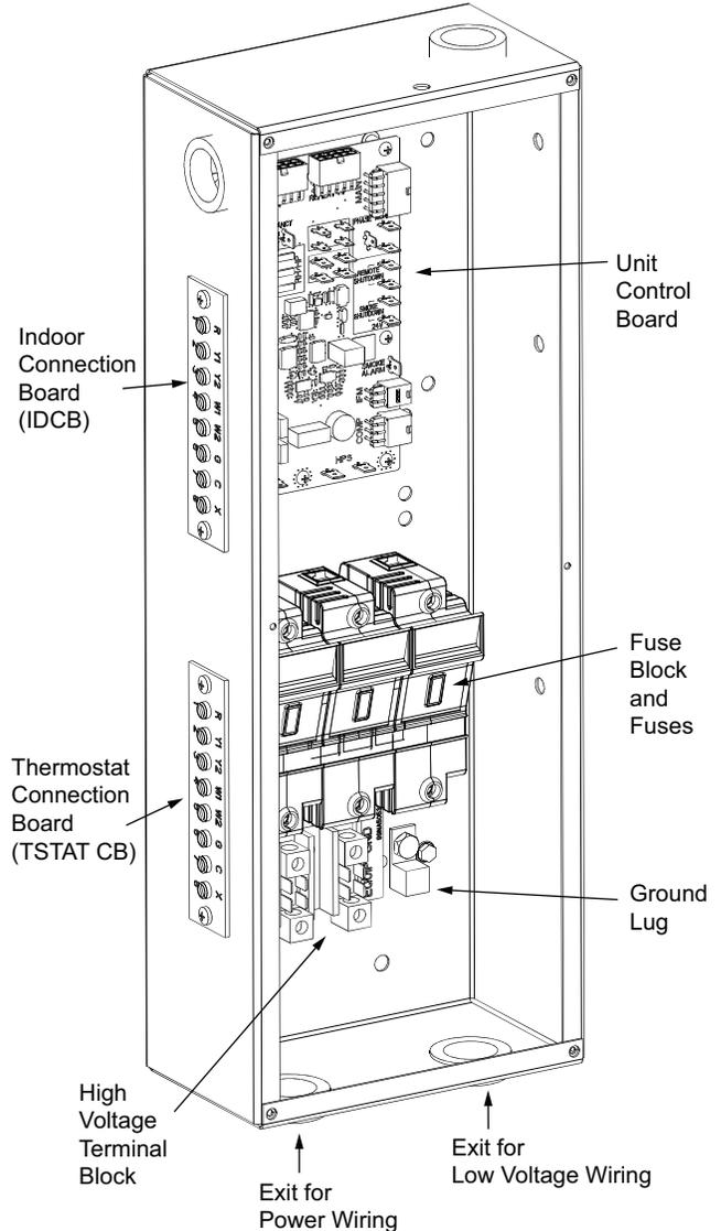
**Fig. 13 — Control Box (Cover Removed) (Typical)**
