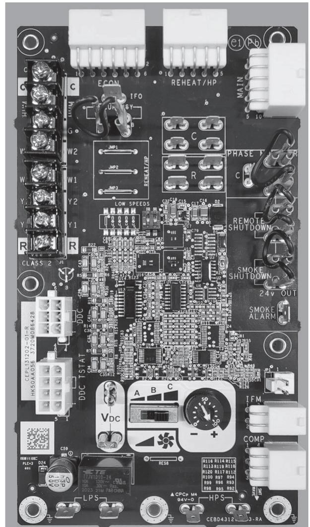
**Fig. 24 — Unit Control Board**
