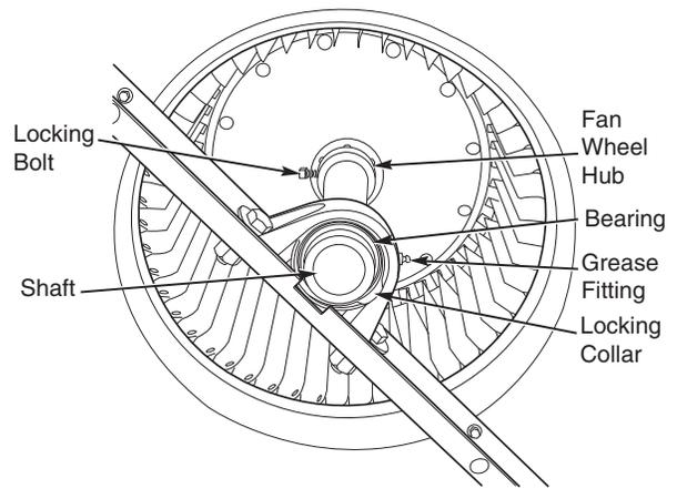
Fig. 25 — Fan Shaft, Bearings, and Fan Wheel (Typical)
