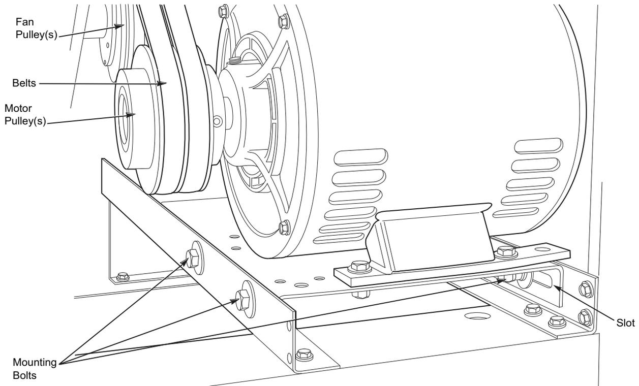
**Fig. 27 — Fan Motor Mounting**
