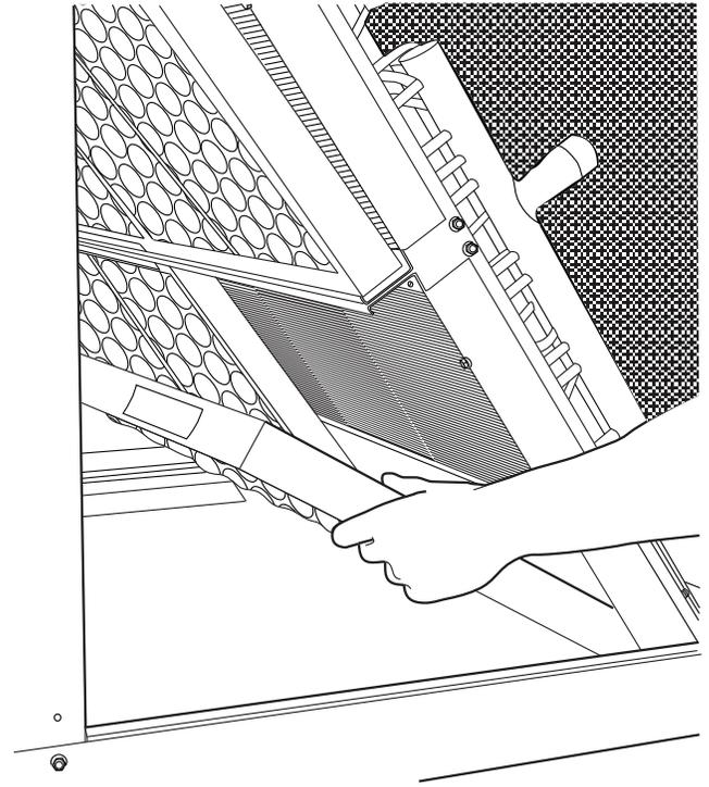
Fig. 37 — Filter Removal/Replacement
