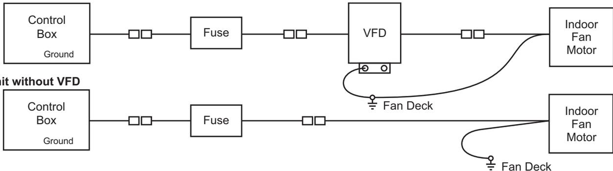
Fig. 35 — To Bypass VFD
