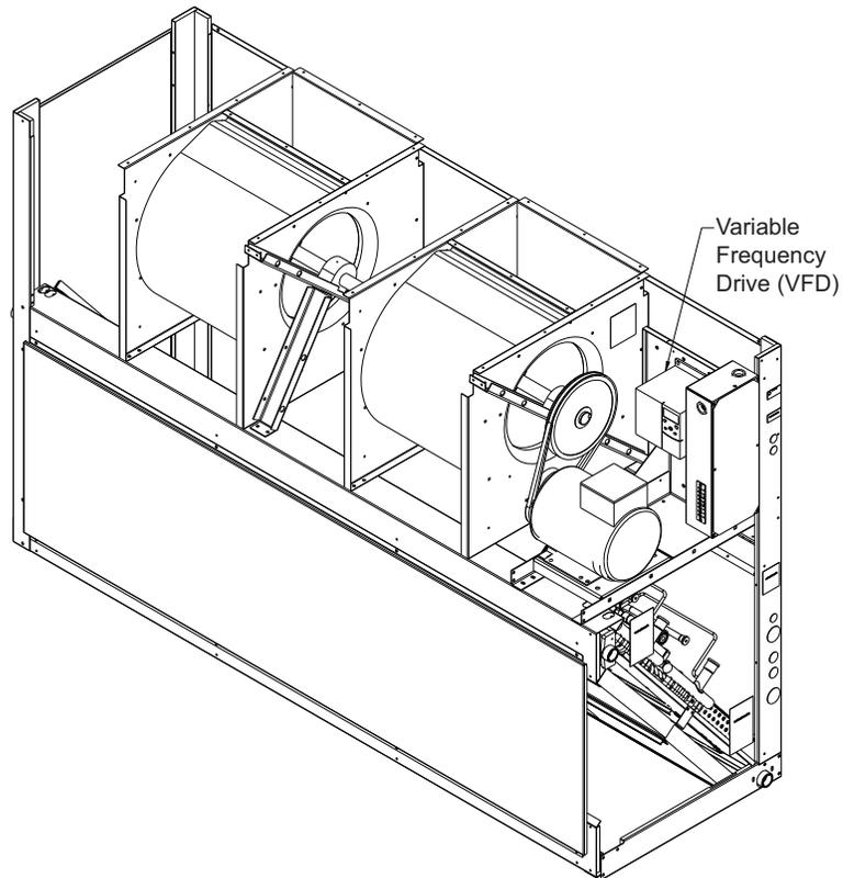
**Fig. 18 — ACS320 VFD Location for the following units: FAS150/180, FHS180 (208/230V and 460V only)**
