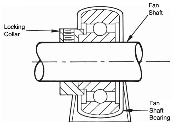
Fig. 26 — Fan Shaft Bearing
