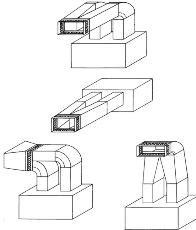
**Fig. 20 — Typical Fan Discharge Connections for Multiple Fan Units**
