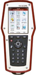
The TA Series 734 SCOPE is a wireless, handheld device for the swift and accurate measurement of differential pressure, flow, temperature and power.
