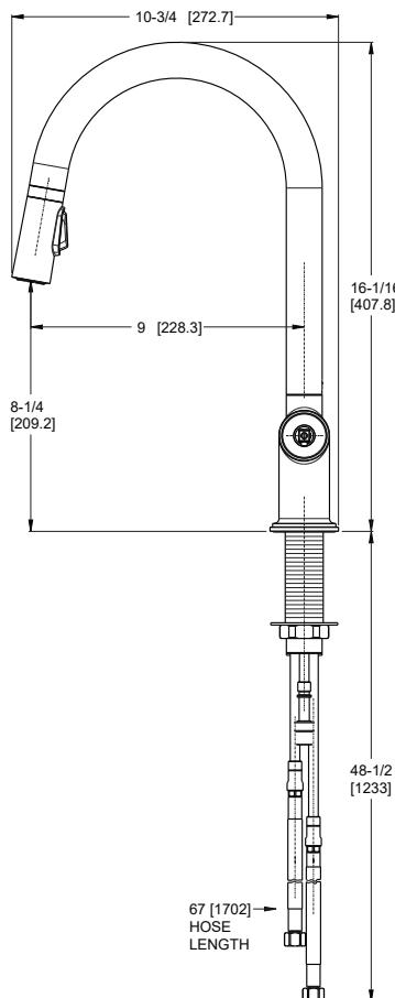
Ø13/8 Min to Ø11/2 Max. Deck Hole Openings
