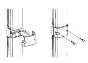
to the wall with appropriate screws. After installing tube, align cover with holes in socket base, and fasten with the stainless steel screws provided.
