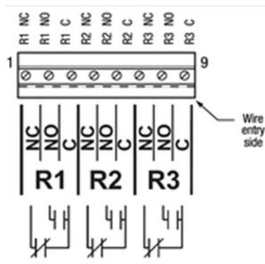
Figure 3-5 Relay Connector
