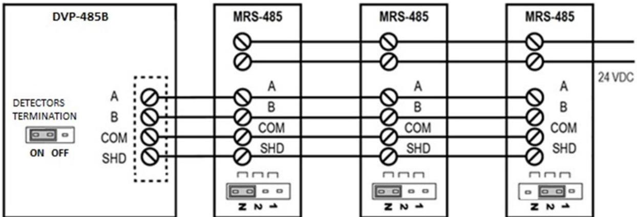
Figure 3-11 EOL Placement greater than 1000 ft
