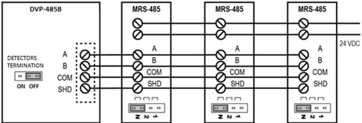
Figure 3-10 EOL Placement Less than 1000 ft
