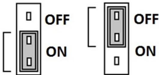
Figure 3-9 End of Line Resistor
