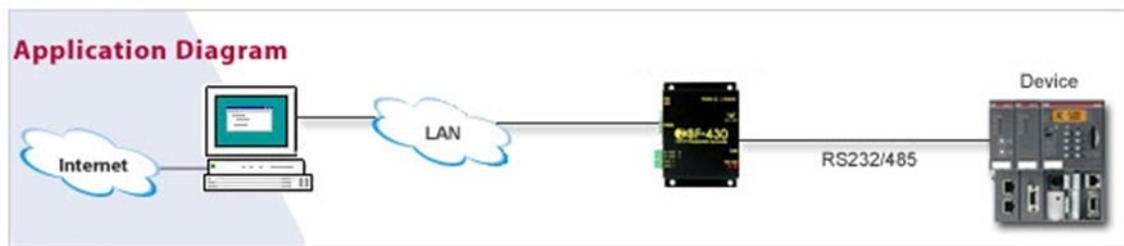
Figure 5-3 RS-485 to Ethernet (TCP/IP)
