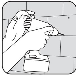
2. Drill holes for screw anchors.
