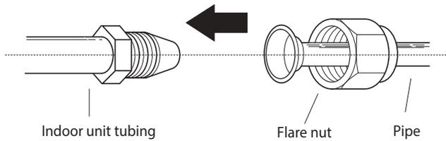
**Fig. 15 — Align the center of the two pipes**
