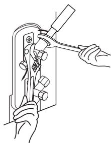
**Fig. 16 — Torque wrench with backup wrench**
