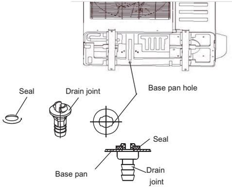
**Fig. 9 —Drain Joint**
