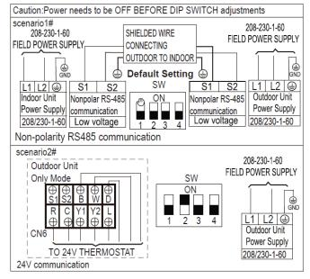
Fig. 24 — Connection Diagram with Ground Terminal
