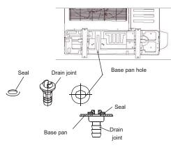
Fig. 11 — Drain Joint
