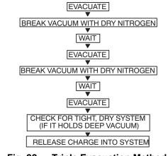
Fig. 22 — Triple Evacuation Method
