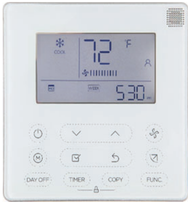
Fig. 34 — Wired Controller KSACN0901AAA
