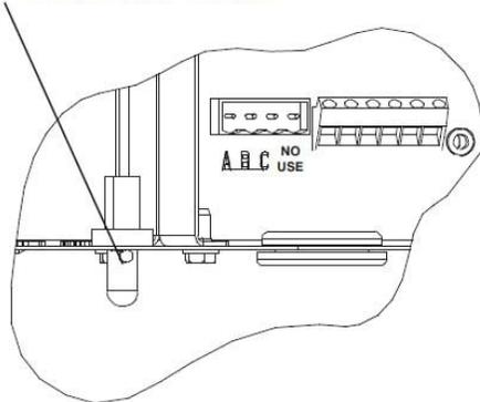
Fig. 45 – Outdoor Air Thermistor (OAT) Attachment
