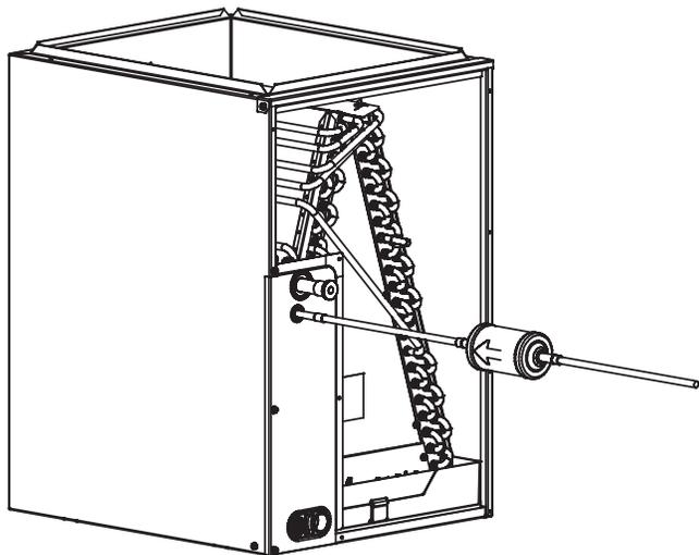
Fig. 24 – Liquid Line Filter Drier - AC
