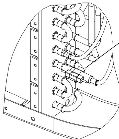
Fig. 46 – Outdoor Coil Thermistor (OCT) Attachment
