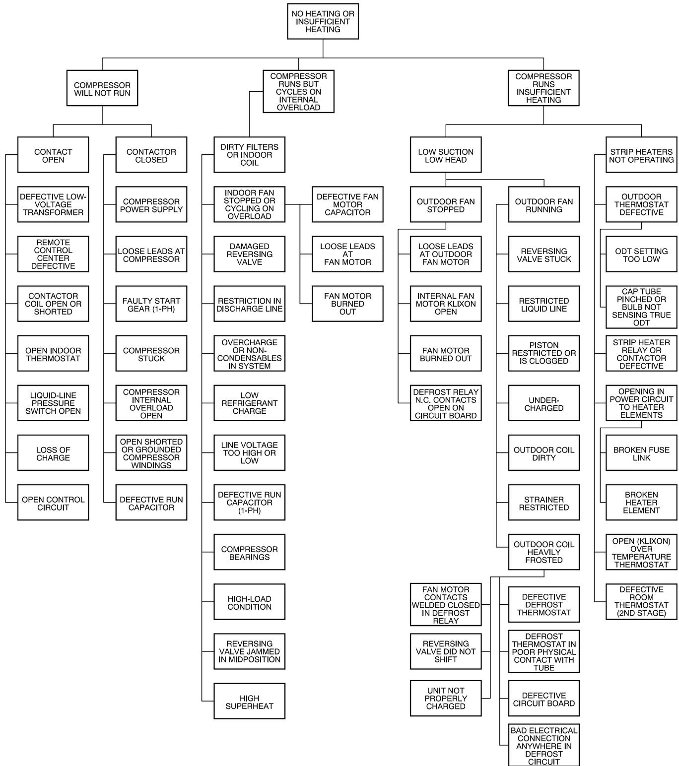
Fig. 49 – Heat Pump Troubleshooting - Heating Cycle
