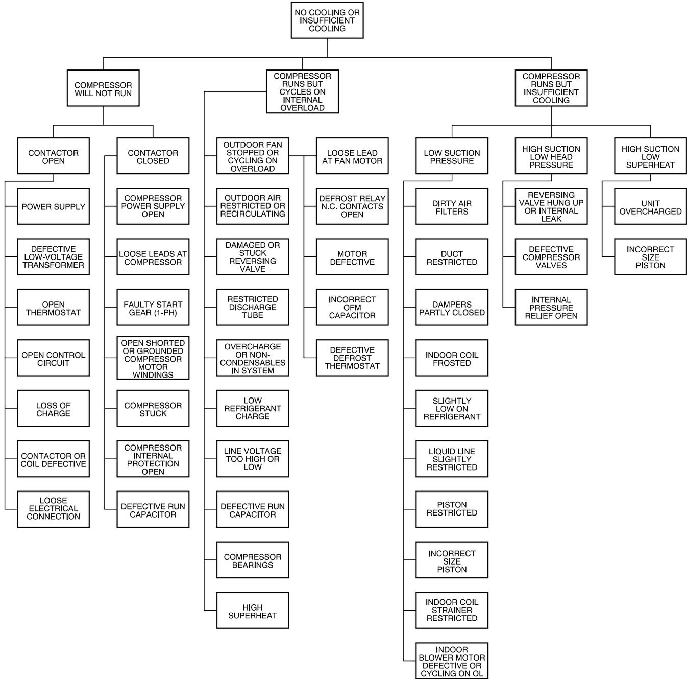
Fig. 50 – Heat Pump Troubleshooting - Cooling Cycle
