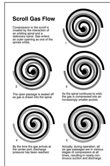
**Fig. 15 – Scroll Compressor Refrigerant Flow**
