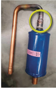
Fig. 2 – Braze Suction Tube to Suction Muffler
