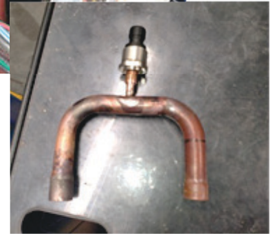
Fig. 11 – Unbraid Suction Tube from Top of Accumulator
