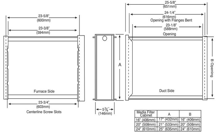
NOTE: Media cabinet is matched to the bottom opening on furnace. May also be used for side return.
