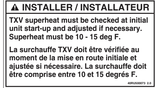
Fig. 20 — TXV Adjustment Label
