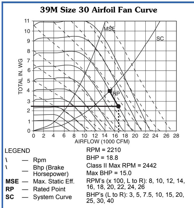
Airflow with a clean filter will be 16,700 cfm. Since airfoil fans are non-overloading (bhp lines run parallel with rpm lines) the bhp does not change (actually, bhp decreases).
