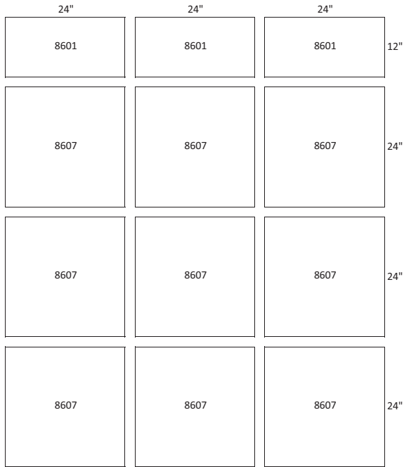
UNIT SIZE: 42T (9) 24" X 24" FILTERS (3) 12" X 24" FILTERS
