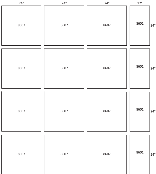
UNIT SIZE 51T (12) 24" X 24" FILTERS (4) 12" X 24" FILTERS
