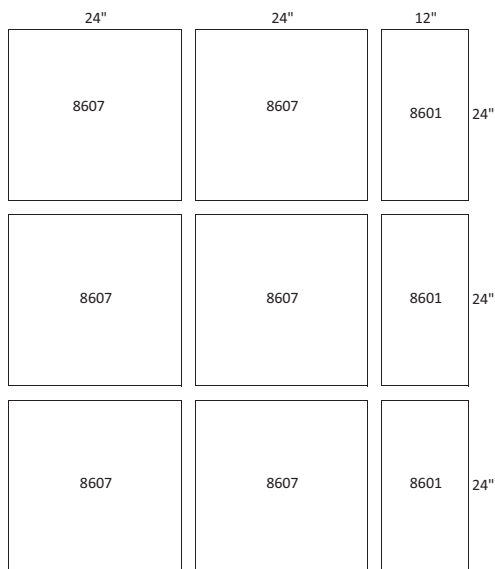
UNIT SIZE: 30T (6) 24" X 24" FILTERS (3) 12" X 24" FILTERS
