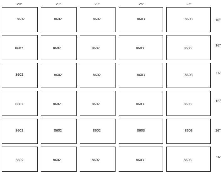
UNIT SIZE: 50W (18) 16" X 20" FILTER (12) 16" X 25" FILTER
