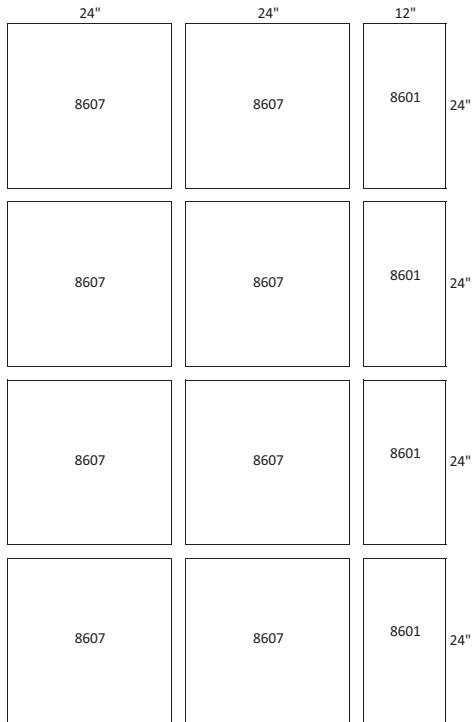
UNIT SIZE: 37T (8) 24" X 24" FILTERS (4) 12" X 24" FILTERS
