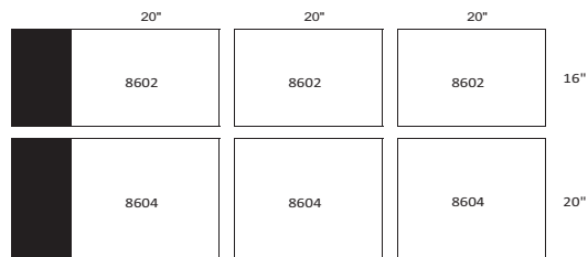
UNIT 14W (3) 16" X 20" FILTER (3) 20" X 20" FILTER
