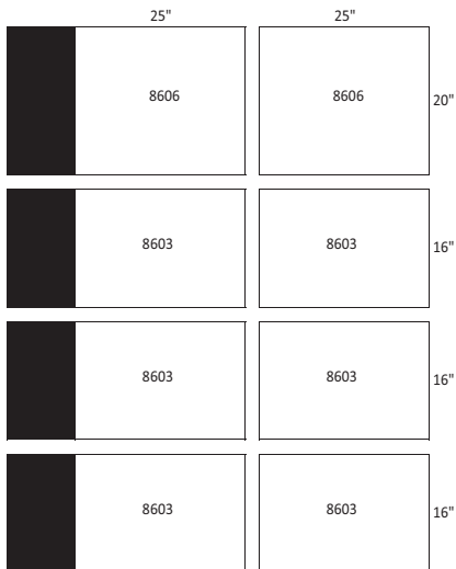
UNIT SIZE: 22T (2) 20" X 25" FILTERS (6) 16" X 25" FILTERS
