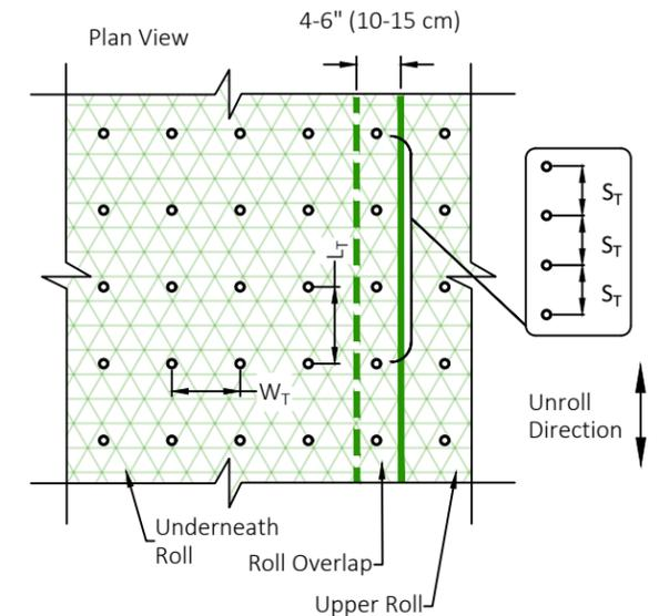
• Pin / Staple / Twist Pin, as appropriate for field conditions
