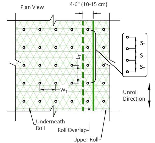
• Pin / Staple / Twist Pin, as appropriate for field conditions
