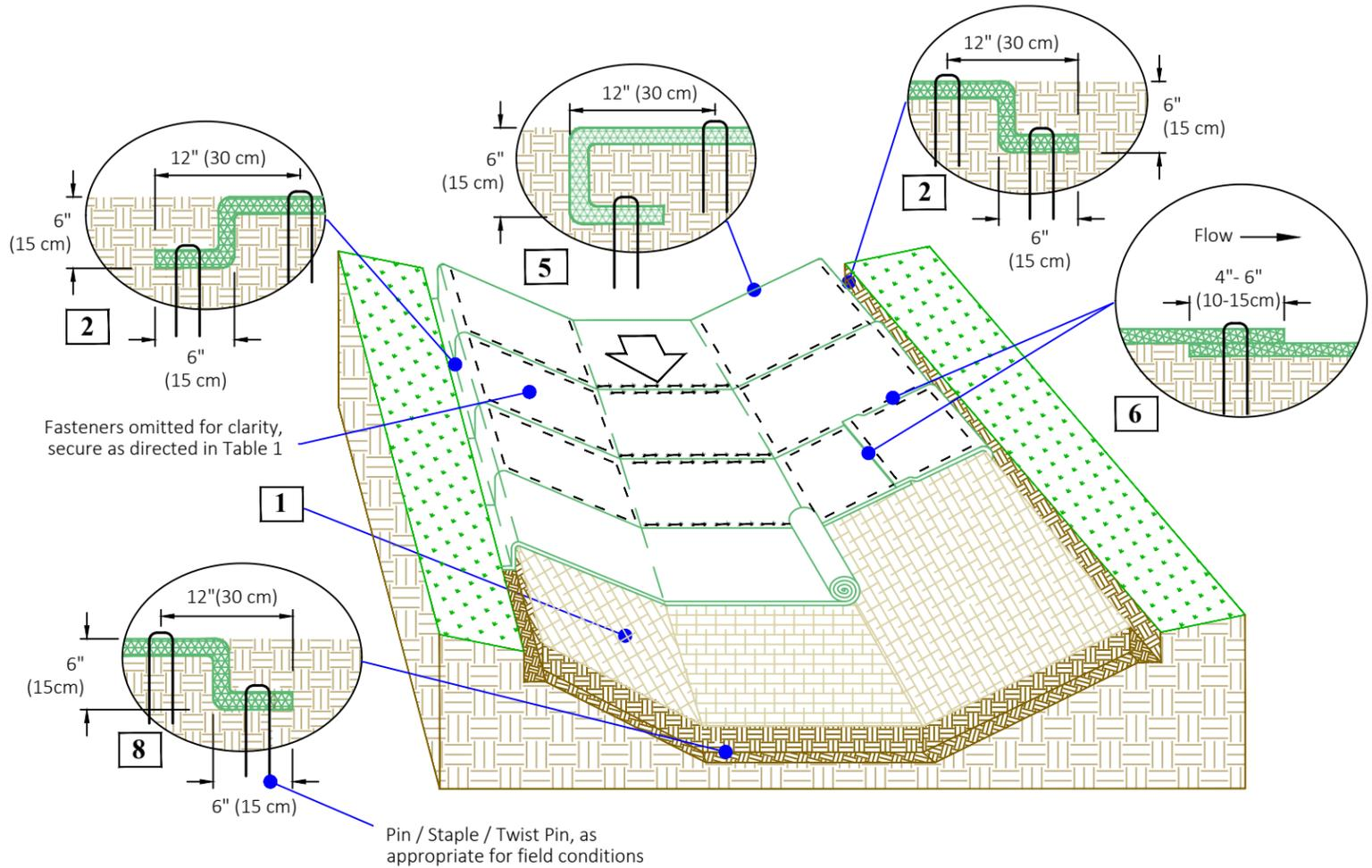
1. Prepare soil (fig. 1) before installing rolled erosion control products (RECPs), including any necessary application of lime, fertilizer, and seed. Ground surface must be free of debris, rocks, clay clods and raked smooth sufficient to allow intimate contact of the RECP with the soil over the entirety of the installation. Apply seed and amendments to the compacted soil.
