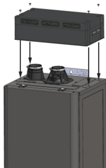
Figure 27 - Outdoor Vent Cap secure with screws.
