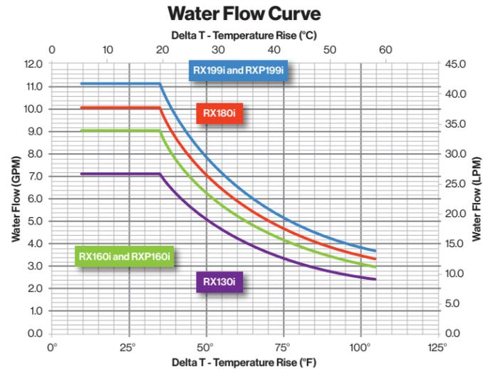
Note: Maximum flow rates may vary based on set temperature, Delta T and altitude
