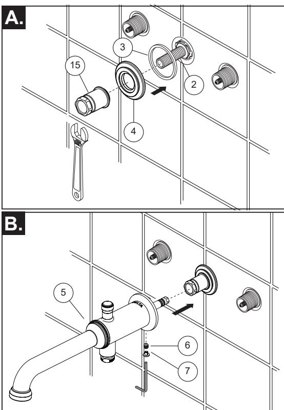
**A.** Install spout flange (4) and gasket (3). **Option:** If mounting surface is uneven, apply suitable sealant to the back surface of gasket, according to the manufacturer's instructions. Finished wall thickness can vary from 1/8" to 1 1/8". Screw mounting nut (15) to the spout shank (2) and tighten it with wrench.
