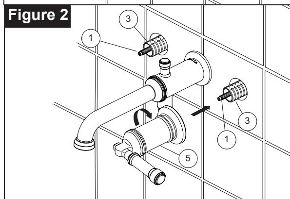
**NOTE:** When drilling holes for hot and cold end valves, the hole size must be between 1 1/2" (38mm) and 1 5/8" (41mm).
