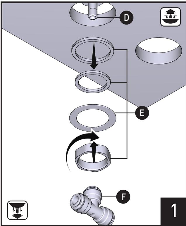
Install Spout **(D)** into sink hole. Install Mounting Hardware **(E)** & Tee **(F)** to secure to sink.
