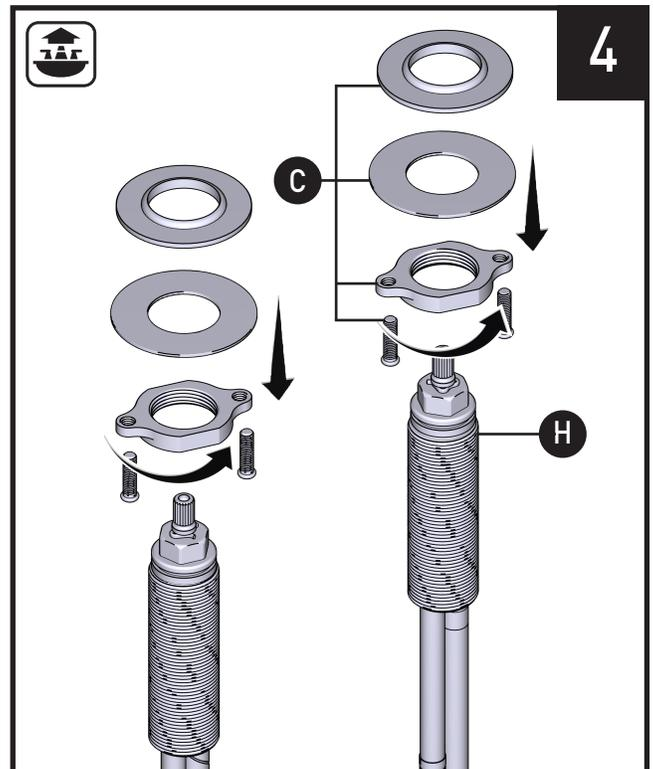
Install Below Deck Mounting Hardware (x2) **(C)** to the Valve Body (x2) **(H)**
