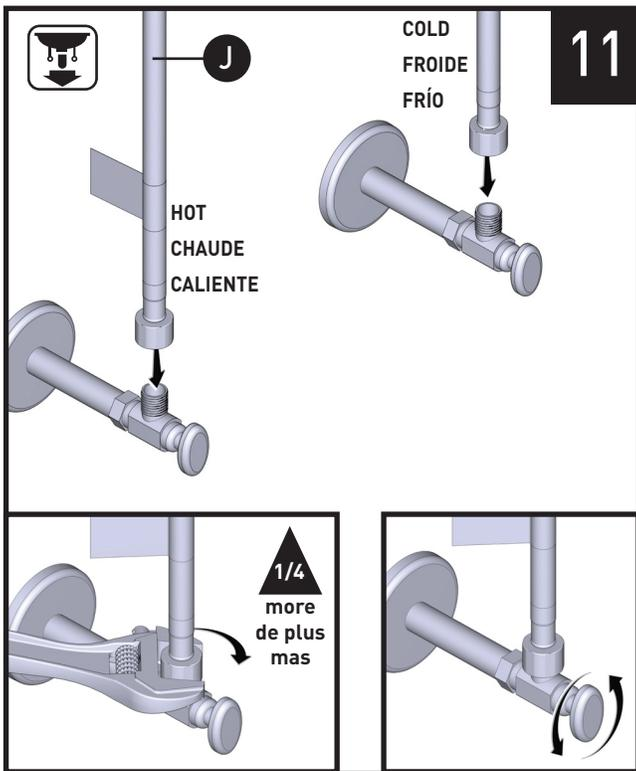
Attach hot & cold supply lines (J) to shut off valves. Tighten by hand, then 1/4 turn more with adjustable wrench. Turn on water and check for leaks.
