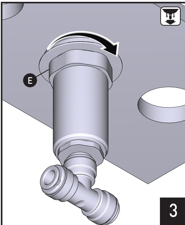
Tighten nut of Mounting Hardware **(E)** with an adjustable wrench.
