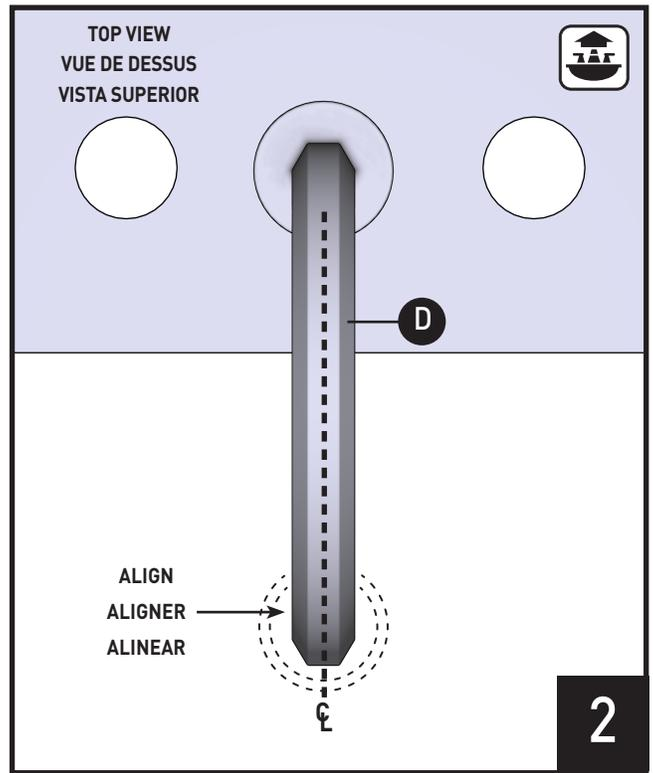
Align Spout **(D)** to center of drain hole as shown.
