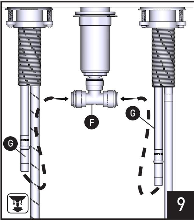
Connect widespread hose (G) from valve bodies into tee (F) as shown. Push in as far as possible for full engagement.
